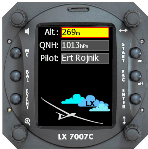
Airfield elevation setting and pilot selection
